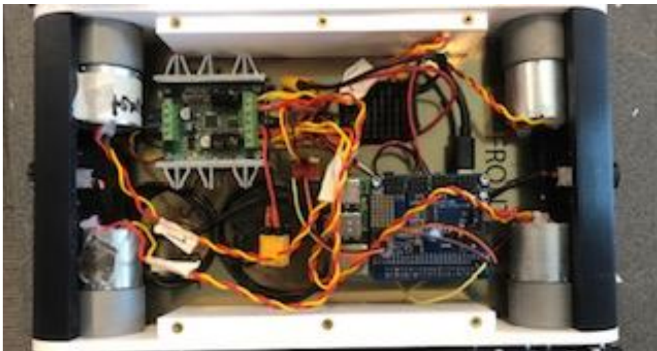
Figure 7 – New Control System for Nibbler robot
