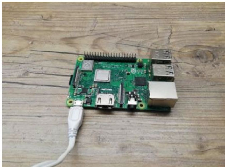
Figure 19: Connection of power supply to Raspberry Pi
